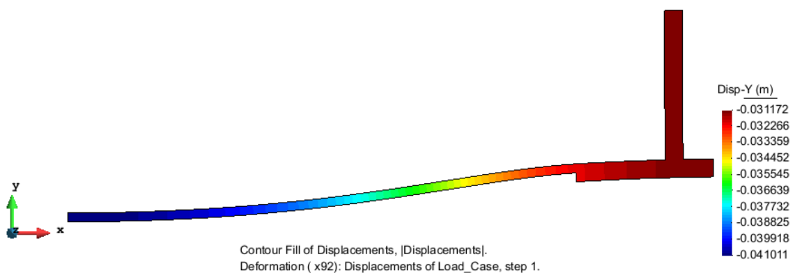
Figure 5: Tank u_y displacement
