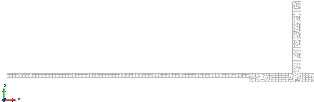
Figure 4: 1.1K nodes converged mesh
