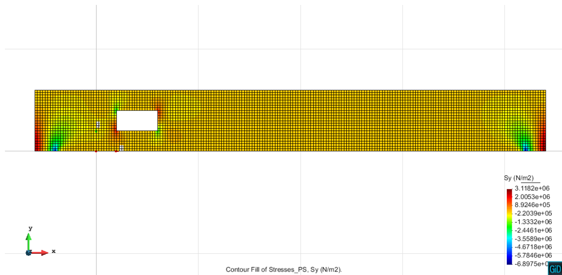
Fig.3.2: Stress (Sx) (N/m²) in the reinforced plate
