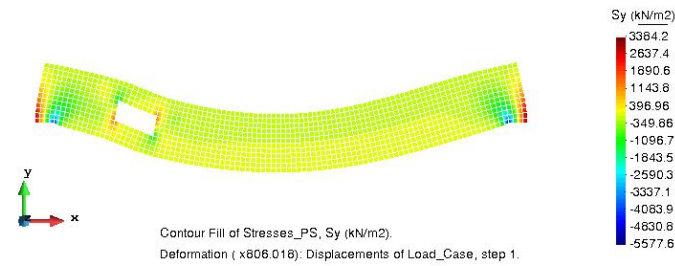
(a) Case 1: without metal reinforcement sheet
