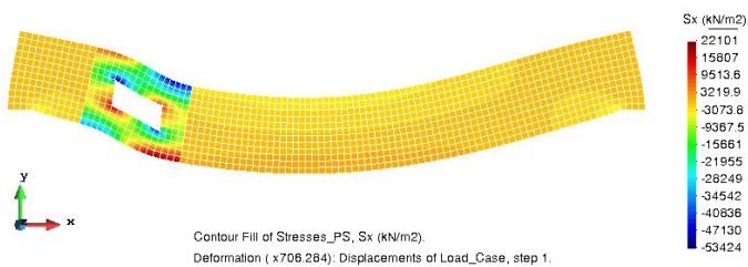
(b) Case 2: with metal reinforcement sheet
