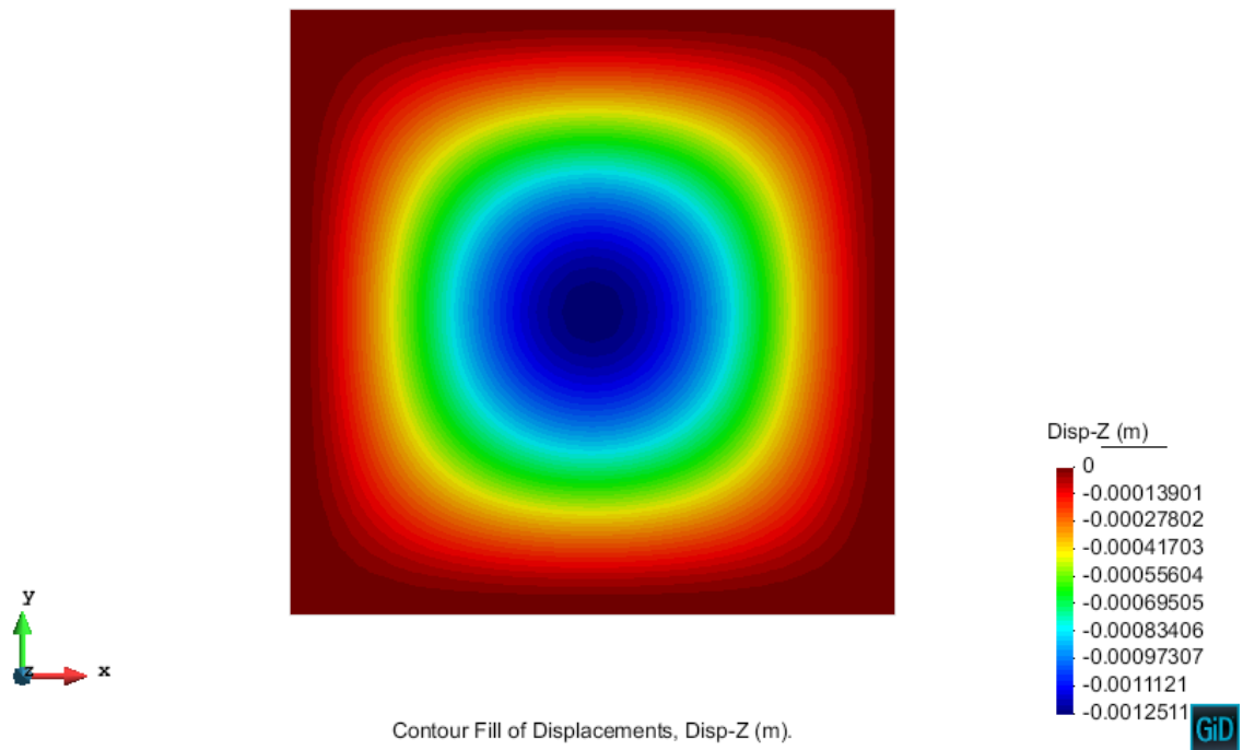
Figure 1.24: Vertical displacements on the plate when analyzed with the RM quadrilateral element.
