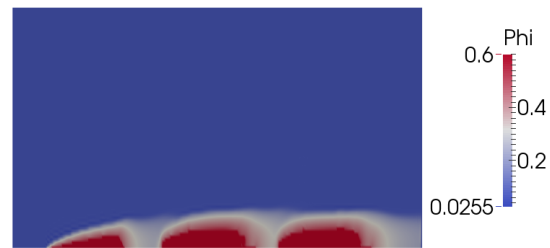
(A) Concentration distribution for the membrane with interspaces along its length which are separated by solid walls
