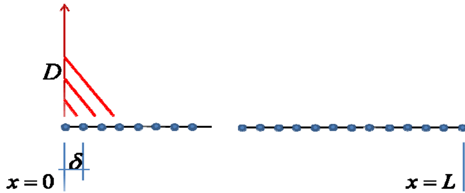
Figure21. Shows the finite element Discretization of the bar for level set approach and the damage function growth.
