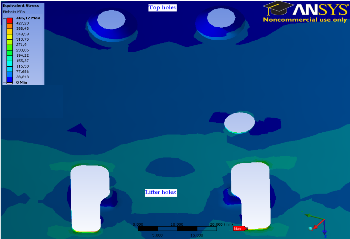
Figure 6.5: Location of maximum Von Mises stress.
