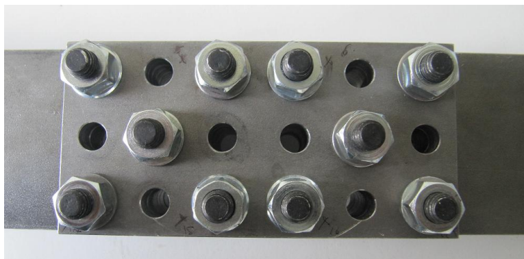
Figure 5.8.: Real System of Bolt Position Type D
