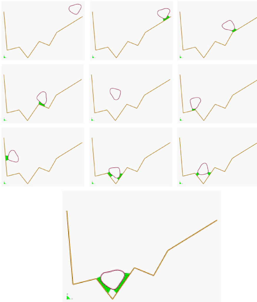
Fig. 13. Bumping of a ball within a container. The layer of contact elements is shown at each contact instant.
