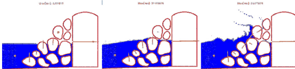
Fig. 25. Detail of the impact of a wave on a breakwater. The arrows indicate the water force on the rocks at different instants.
